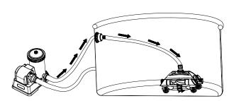
1. Turn off the filter pump. From inside of the pool, unscrew the nozzle from the water return connector. See Fig. 1.
