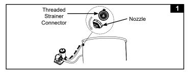
Make sure the micro-screen (6) is inside the hose adaptor (7), then screw the hose adaptor to the threaded strainer connector, from inside of the pool. See Fig. 2.
