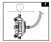
8. Turn on the filter pump and make sure water is flowing through the micro-screen (6) and the hose adaptor (7). The auto cleaner is now moving and vacuuming the pool floor. See Fig. 8.
