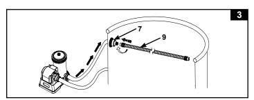
**4.** Extend the hose **(9)** to the opposite side of the pool wall so that it over hang the wall and cut the excess hose with a scissor, refer to below table and fig 4.
